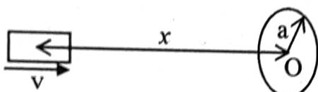
A small bar magnet of dipole moment  $M$  is moving with speed  $v$  along  $x$  direction towards a small closed circular conducting loop of radius ' $a$ ' with its centre  $O$  at  $x = 0$  (see figure). Assume  $x \gg a$  and the coil has a resistance  $R$ . Then which of the following statement(s) is/are true ?
