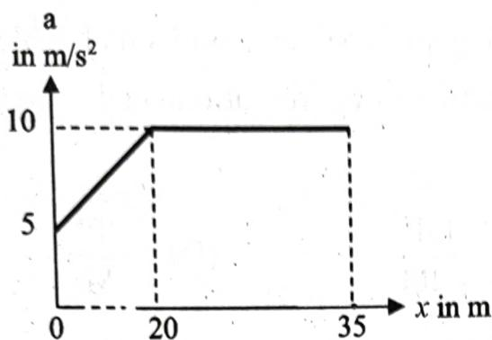
The acceleration vs distance graph for a particle moving with initial velocity  $5 \text{ m/s}$  is shown in the figure. The velocity of the particle at  $x = 35 \text{ m}$  will be
