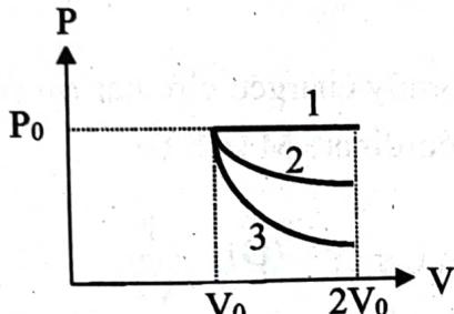
In the given figure, 1 represents isobaric, 2 represents isothermal and 3 represents adiabatic processes of an ideal gas. If  $\Delta U_1$ ,  $\Delta U_2$ ,  $\Delta U_3$  be the changes in internal energy in these processes respectively, then
