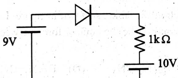
What is the value of current through the diode in the circuit given?
